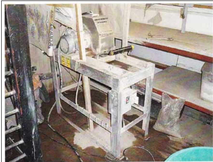
Core splitting facilities – Diamond saw (B. Solano, 2009)
