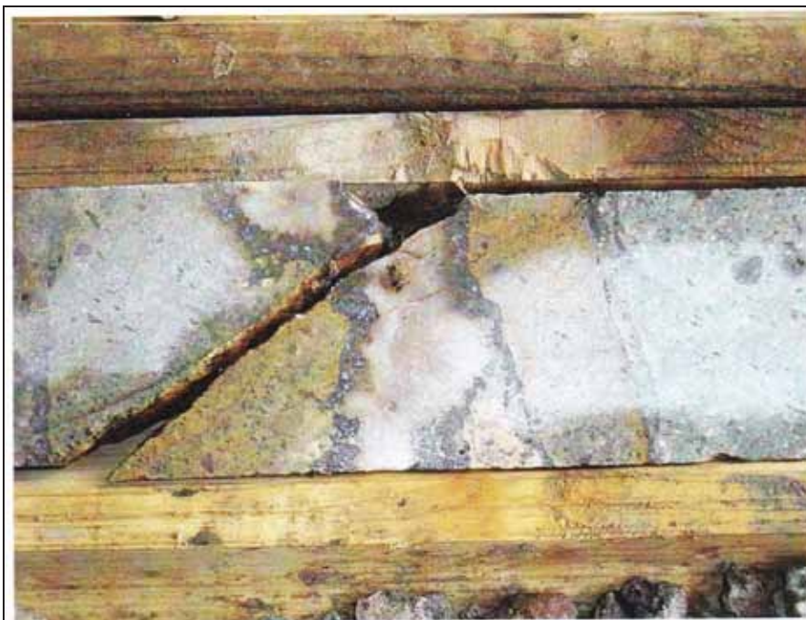
Half core sample split (B. Solano, 2009)
